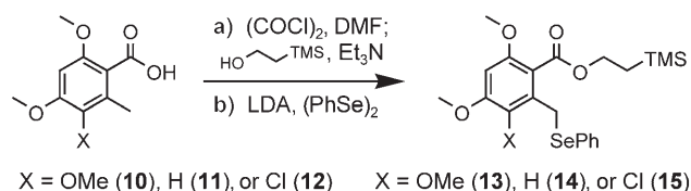
Scheme 3. Synthesis of aromatic moieties 13–15 . a) (COCl) 2 , (1.0 equiv), DMF (cat.), CH 2 Cl 2 , 0 °C, 1 h, then 2-(trimethylsilyl)ethanol (1.0 equiv), Et 3 N (2.6 equiv), 4-DMAP (cat.), 23 °C, 1 h, 96–98%; b) LDA (2.0 equiv), (PhSe) 2 (1.0 equiv), THF, –78 °C, 1 h, 89–91%, 4-DMAP = 4-dimethylamino pyridine, LDA = lithium diisopropylamide, TMS = trimethylsilyl.
